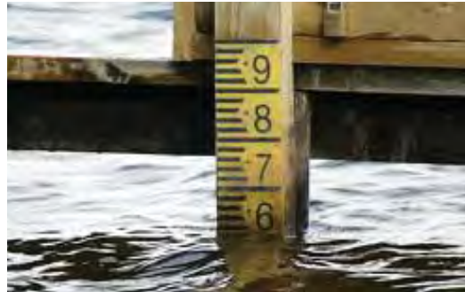
K.1 Water gauge showing water levels
