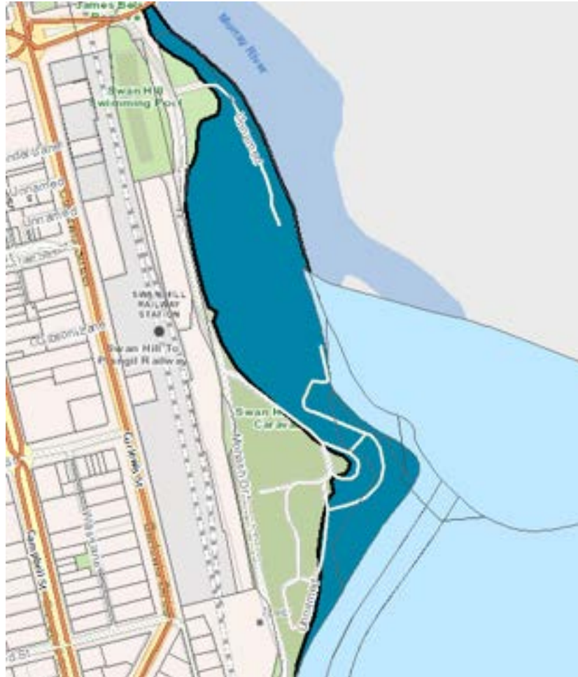
Figure One: Light Blue – Existing LSIO and Darker Blue – Additional land below the 1% AEP flood level
