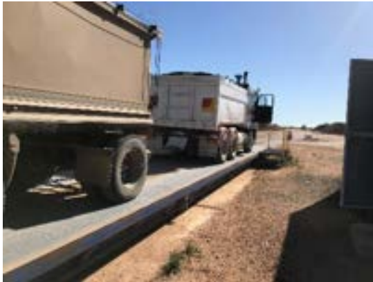
Figure 9 Above ground weighbridge
