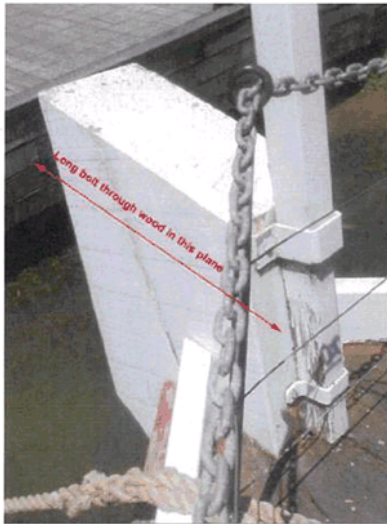
Repairs to Stem Post to reduce cracking
