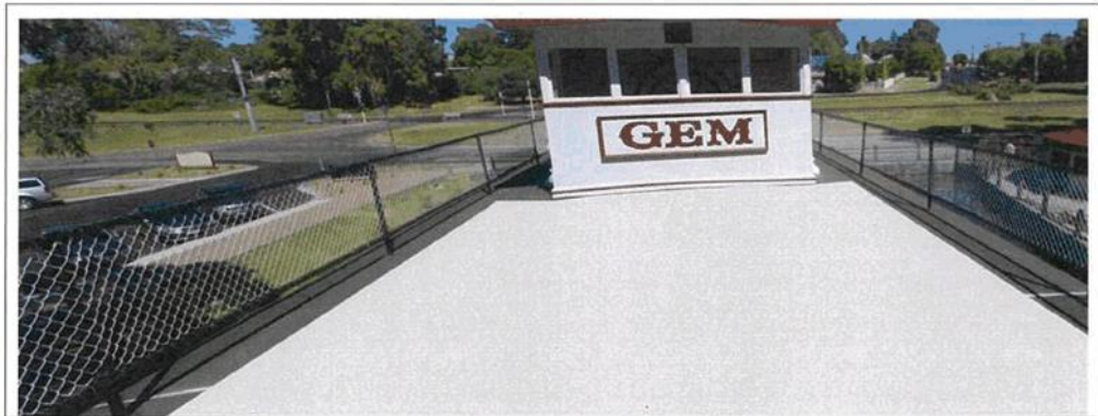
Proposed panel of grey DuroMastic to reduce heat uptake – looking aft
