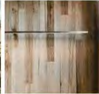
Vic Ash Lining
